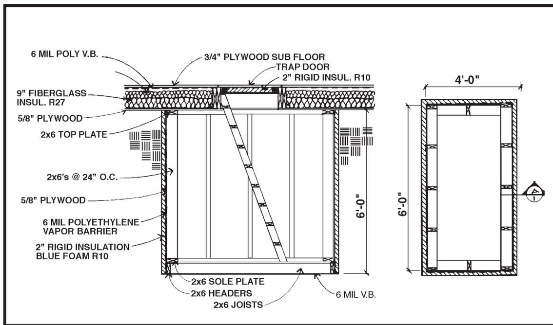
Figure 1. Example blueprint for below floor root cellar.
